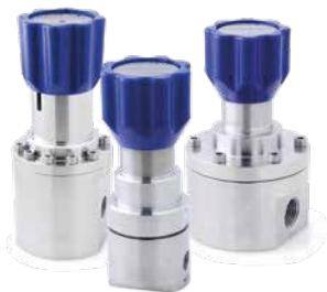
Primarily for gas service. Diaphragm sensed elements control up to 10 bar (145 psi) and piston-sensed elements covering up to 414 bar (6,000 psi). Ports 1/2" to 1".
